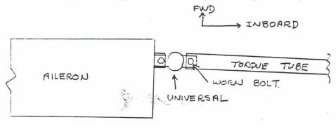
I disassembled the torque tube from the universal joint and was surprised to find that the 3/16" bolt had been significantly worn down in two areas where it passed through the universal joint (See sketch).
