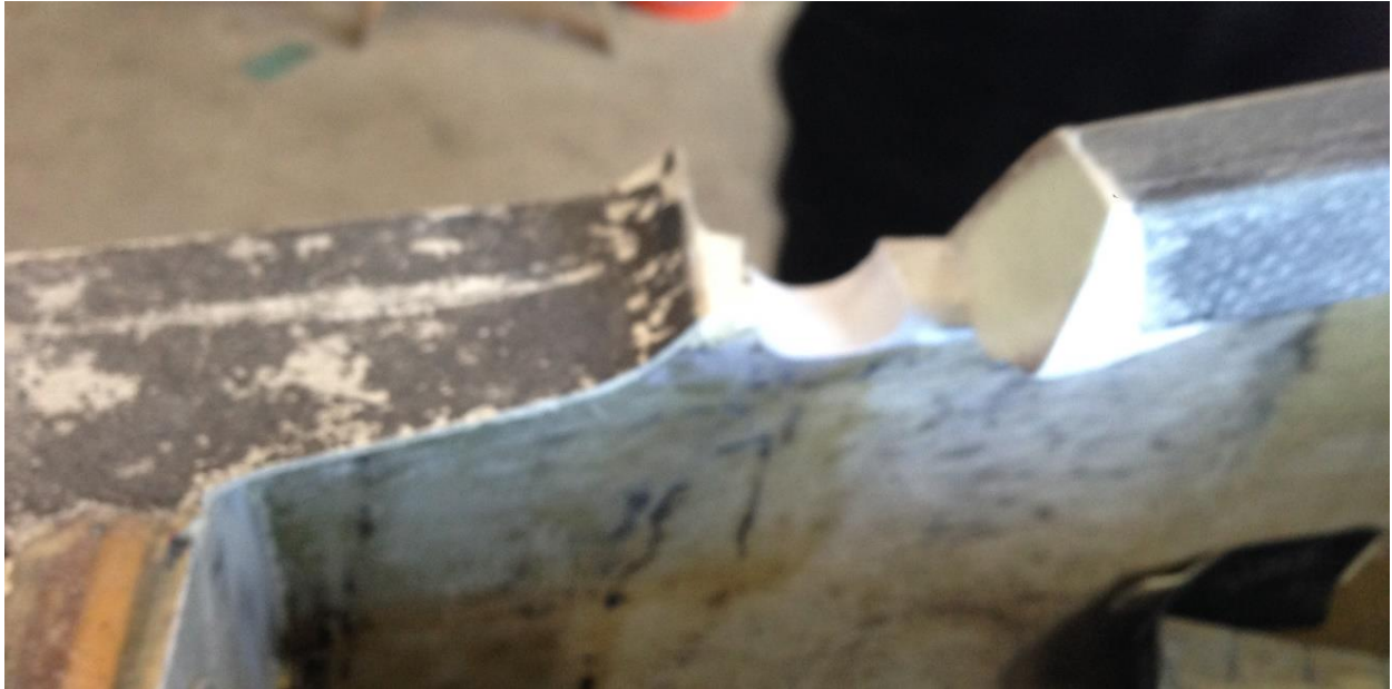
11. The right side of the fuselage, mostly inside skin, longeron to the right, elevator bulkhead to the bottom left, and canard "bed" (worn painted black paint) on the left.
