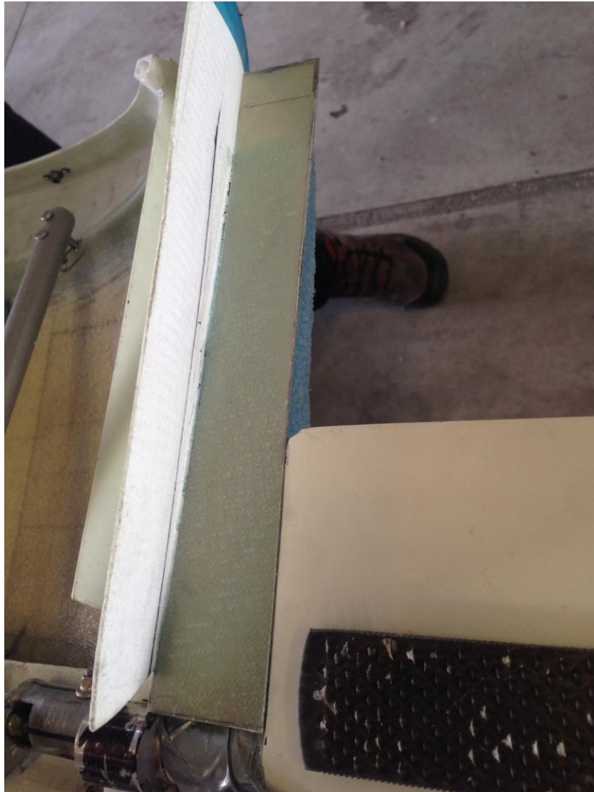
22. The Faux elevator bottom on the right side of the canard/elevator.
