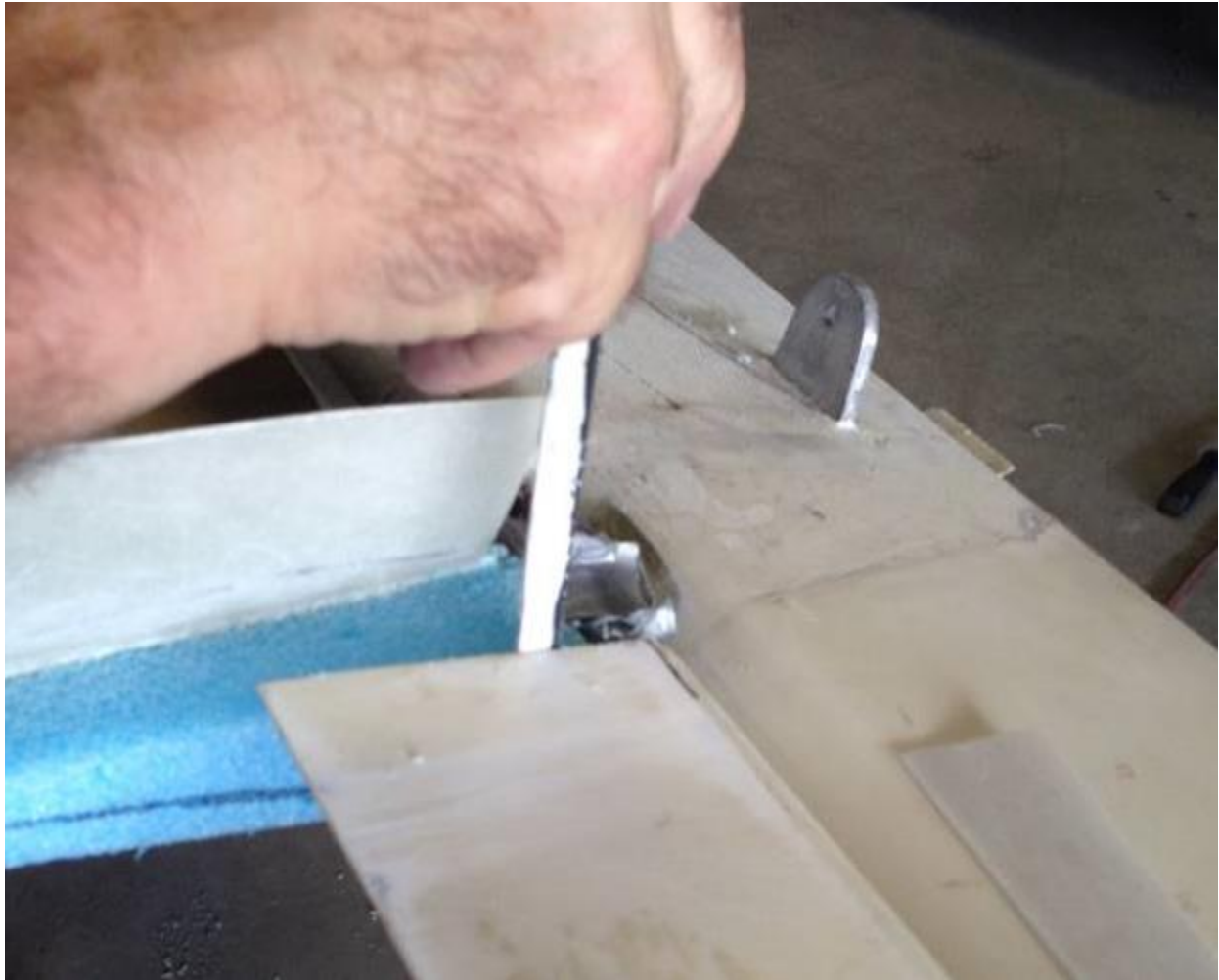
29. Sawing some clearance between faux elevator and elevator.
