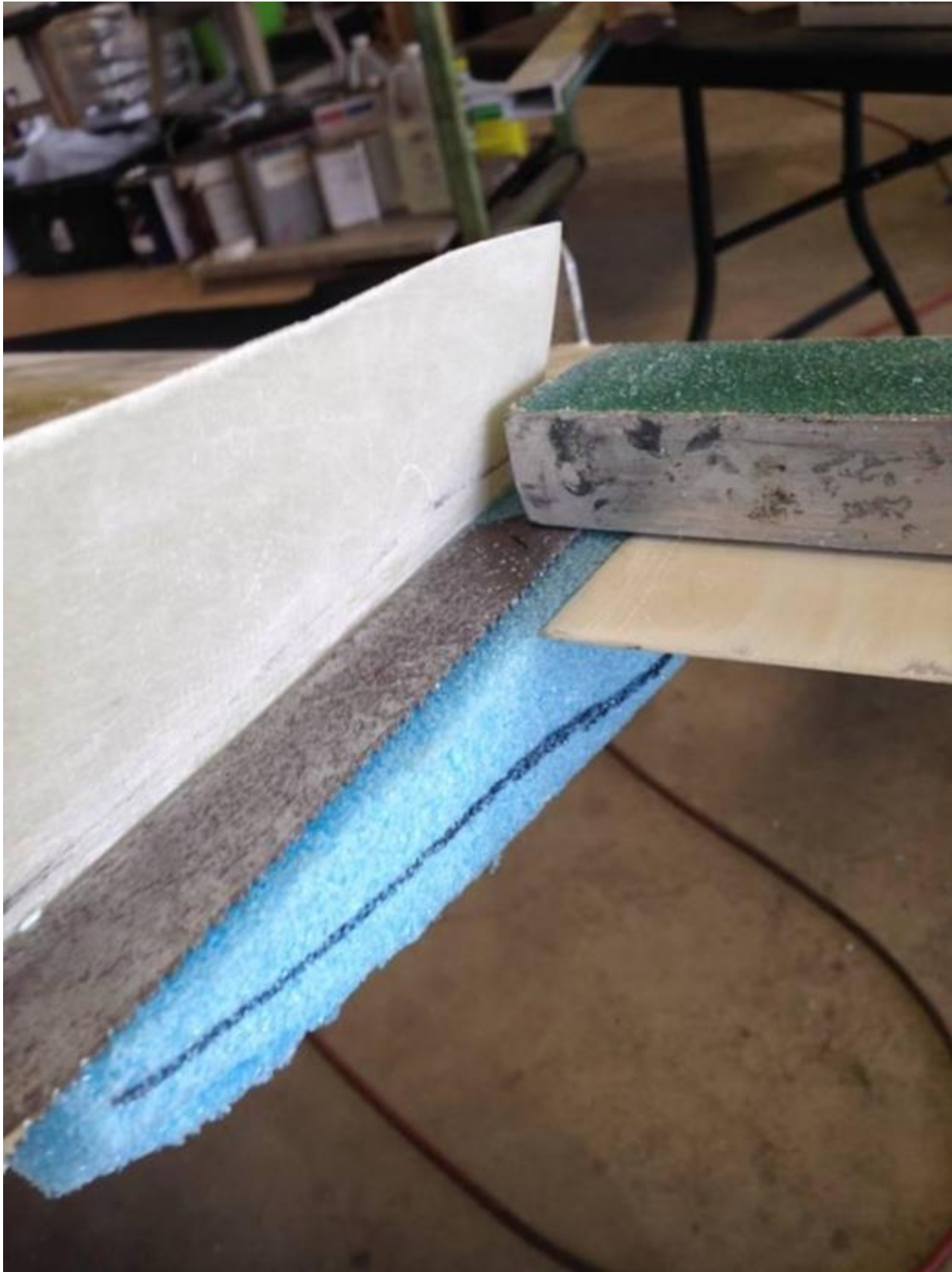
20. Saw blade used as dummy before installing the bottom skin of the left faux elevator.
