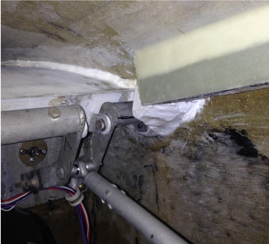
16. Right side bearing in fuselage, longeron front edge filled with micro, upper bearing not so clear to see. Right side saddle is again light green extending to the right side of the photo.
