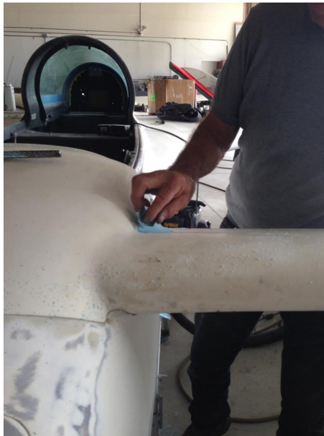
24. Dave used surfoam tools, the \frac{1}{4} circle and a little \frac{1}{2} thick surfoam tube.
