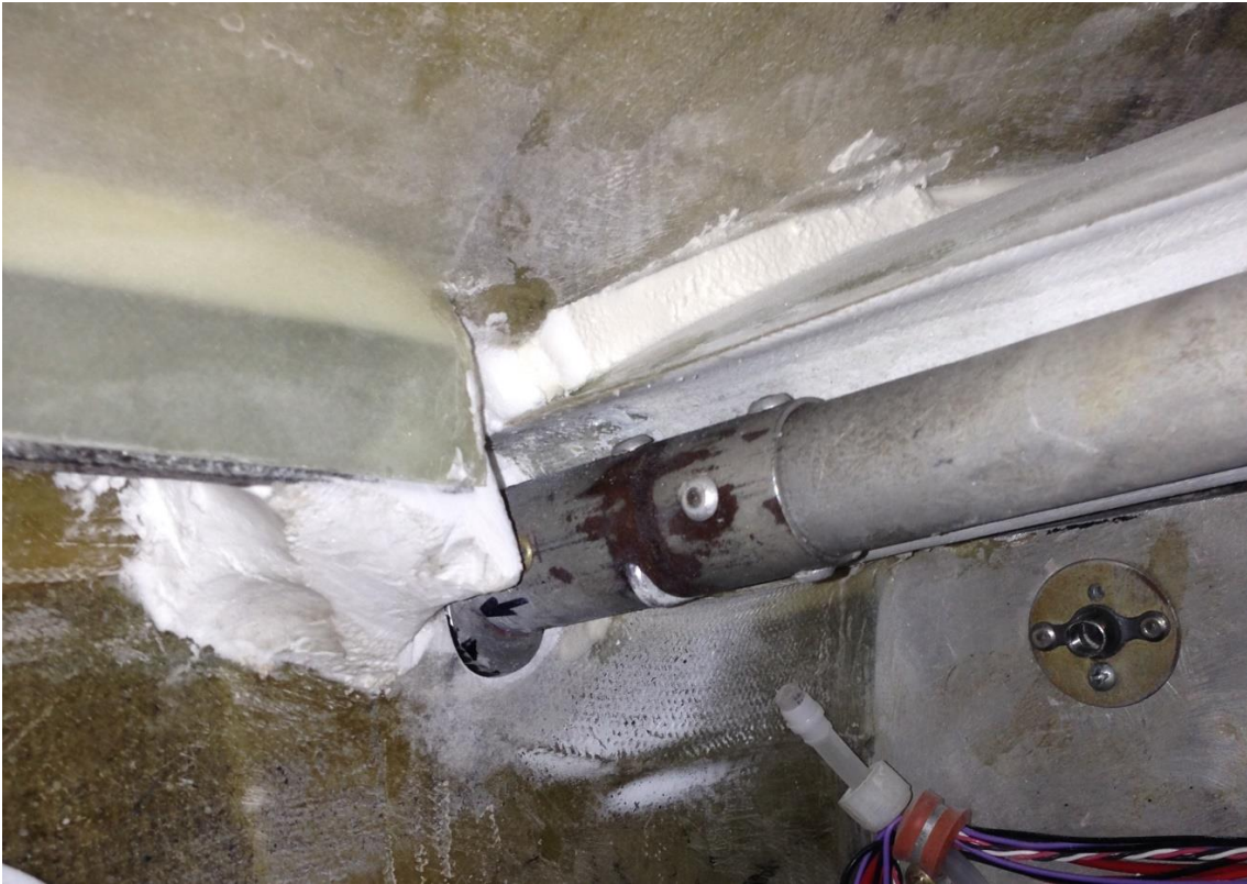
15. Left side upper half of bearing hidden from this angle, the left saddle in green to the left side of the photo, canard bolt nutplate on washer to the right side below the elevator tube.
