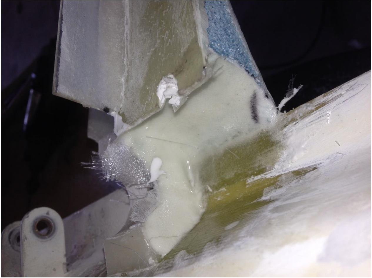
17. Canard off and upside down – fill sanded and 4 oz cloth applied.
