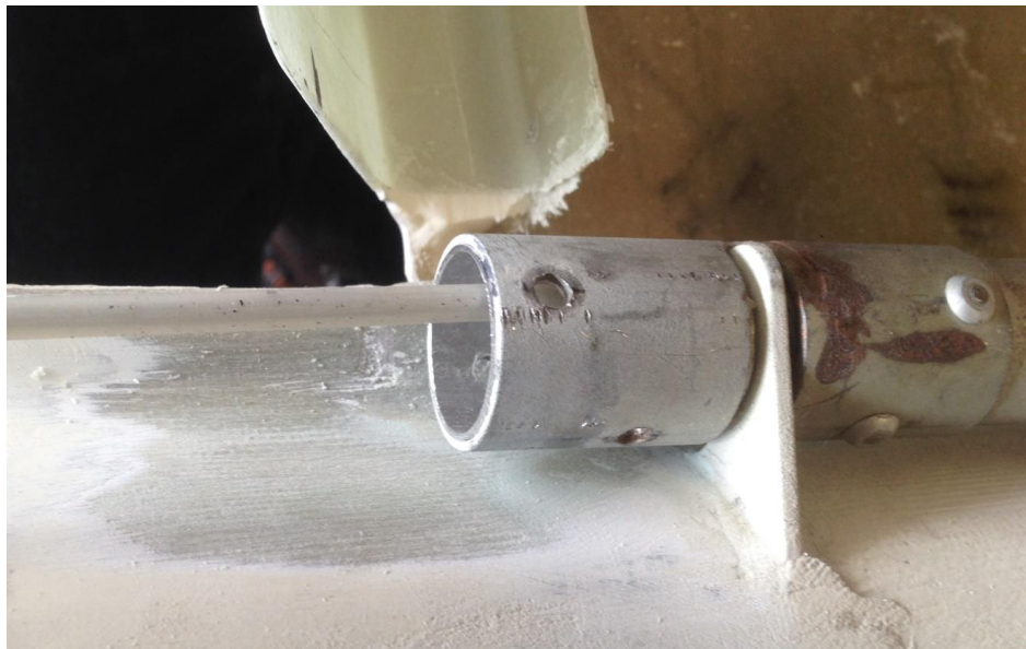
3. The remainder of the internal elevator tube with the steel reinforcement, rivets removed and hinge pin inserted.
