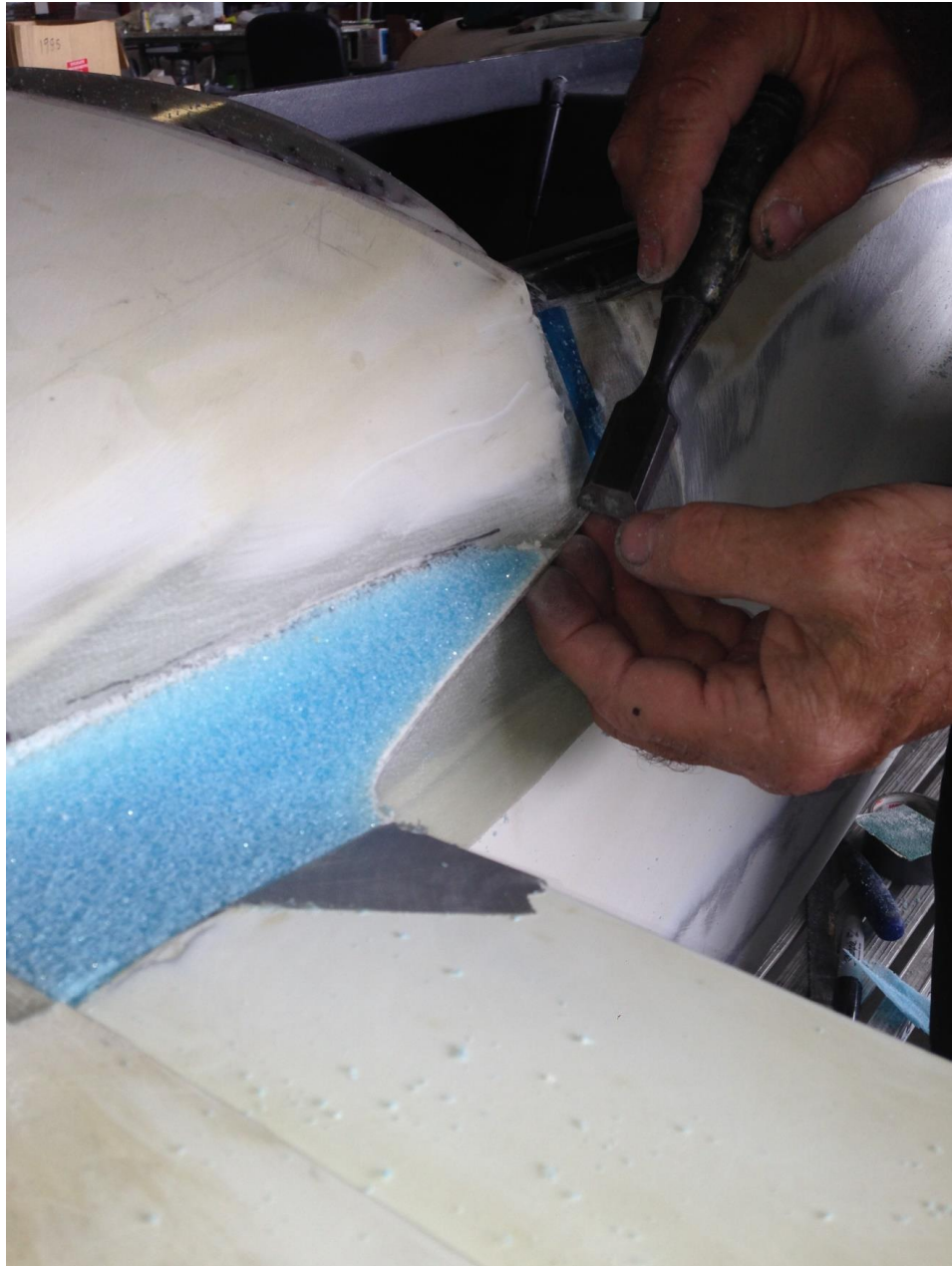
25. A chisel used to make a flox tip.
