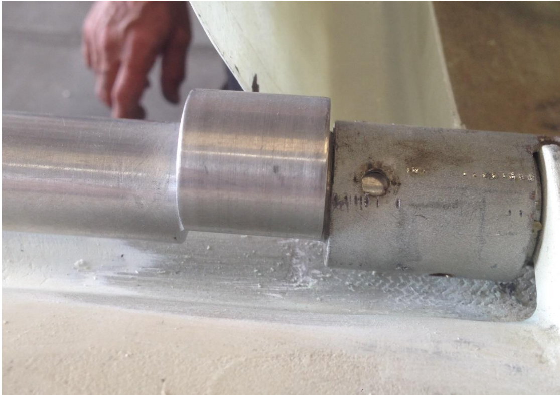
5. The eccentric cut and inserted in the Steel reinforcement.
