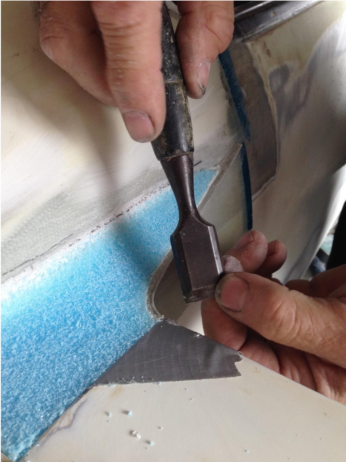
26. Taking out the foam on the trailing edge of the faux elevator.
