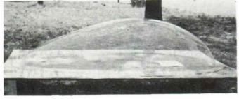
the canopy to rise (12-15 in.). I made a small window in the box to watch the glass and heat, and brought the temperature up to 280 deg. F., then opened the air valve and the canopy began to rise. When the glass reached the height I wanted, I held it with the air valve and opened the door to let it cool."
