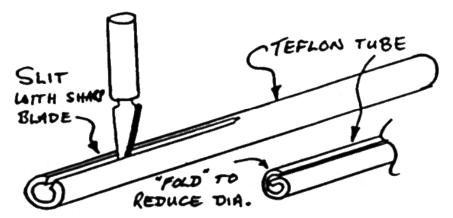
Now fold it up to reduce its diameter, and push it through the hinge. When you have it all the way through, (the unslit half is not into the hinge yet) now insert your welding rod hinge pin into the unslit half of the Teflon tube, then pull the whole works through the hinge until your new hinge pin and Teflon liner are properly aligned in the hinge. Trim off the "slit" portion of Teflon tube and discard.
