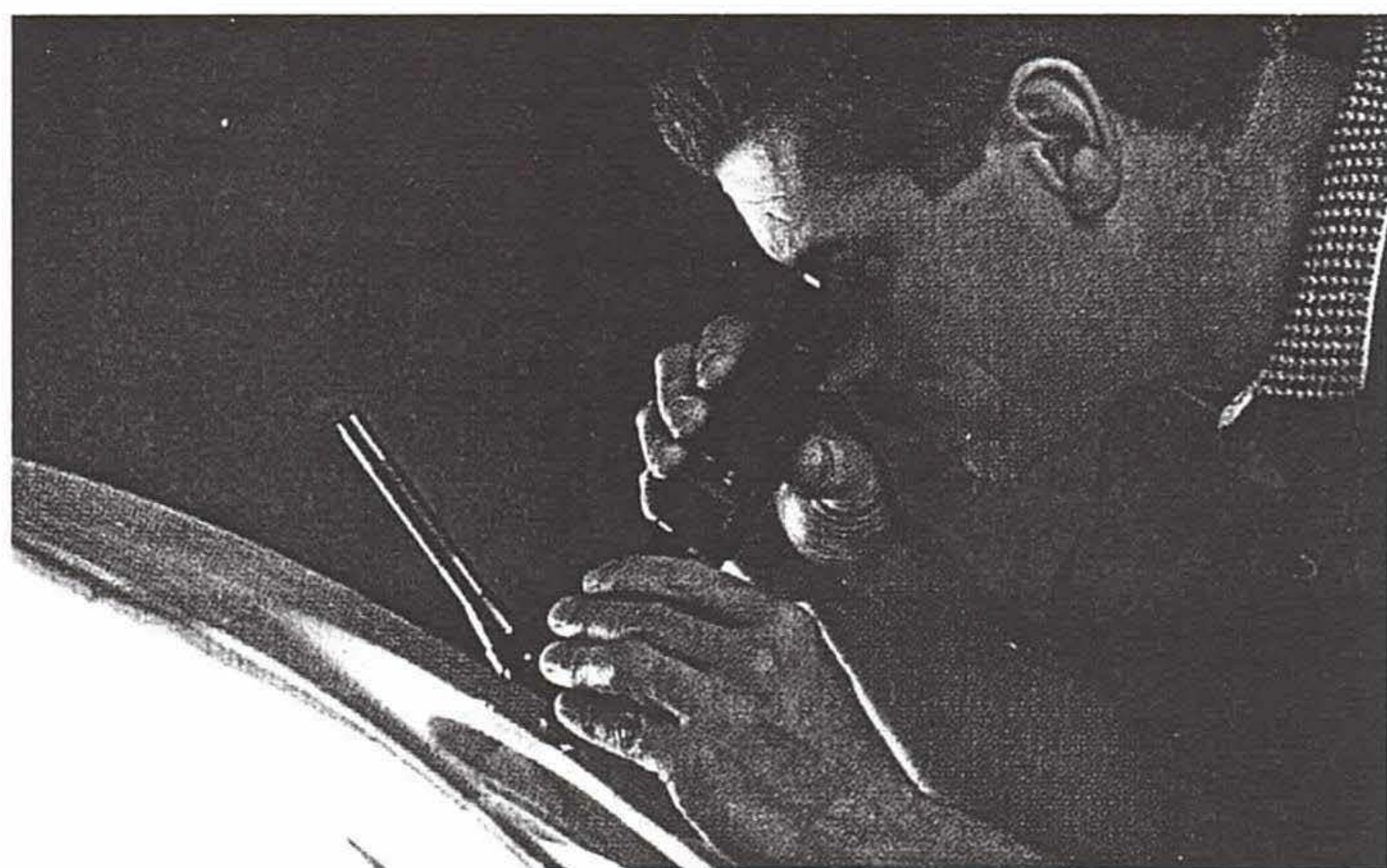
Window repair facilities such as Lee Aerospace in Wichita use high-power optical instruments to determine the depth of scratches and cracks.
