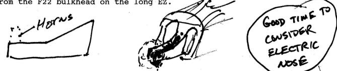
2. Then you either remove and replace the small nose bulkhead with this larger version or build it out to the new dimensions with dense foam.
