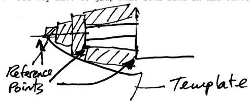
6. Carve the bottom in a nice smooth line, remembering that the nose stop will still need to be the first thing to touch down when you gear up. Further, the closer you get to the original profile under the nose gear, the less fill you will need on the nose gear leg when you are finished. There are some nose gear door plans which are better used if the gear leg is sunken in about .25 inches.
