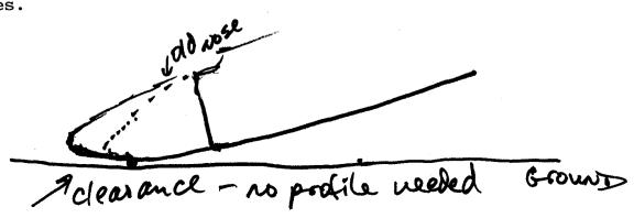
7. Carve the top freehand or using the top template (<u>female</u> template #4) and also keep the notes you have cut off the template to show the profile of the interior of the top of the nose and nose door. Now, the NG31 will either be cut off inside your door or you must make provisions to leave it intact, which I prefer. I suggested you lay silver tape over the top of the NG31 down each side so it does not attach to the nose top when you later cut it off and play with it.
