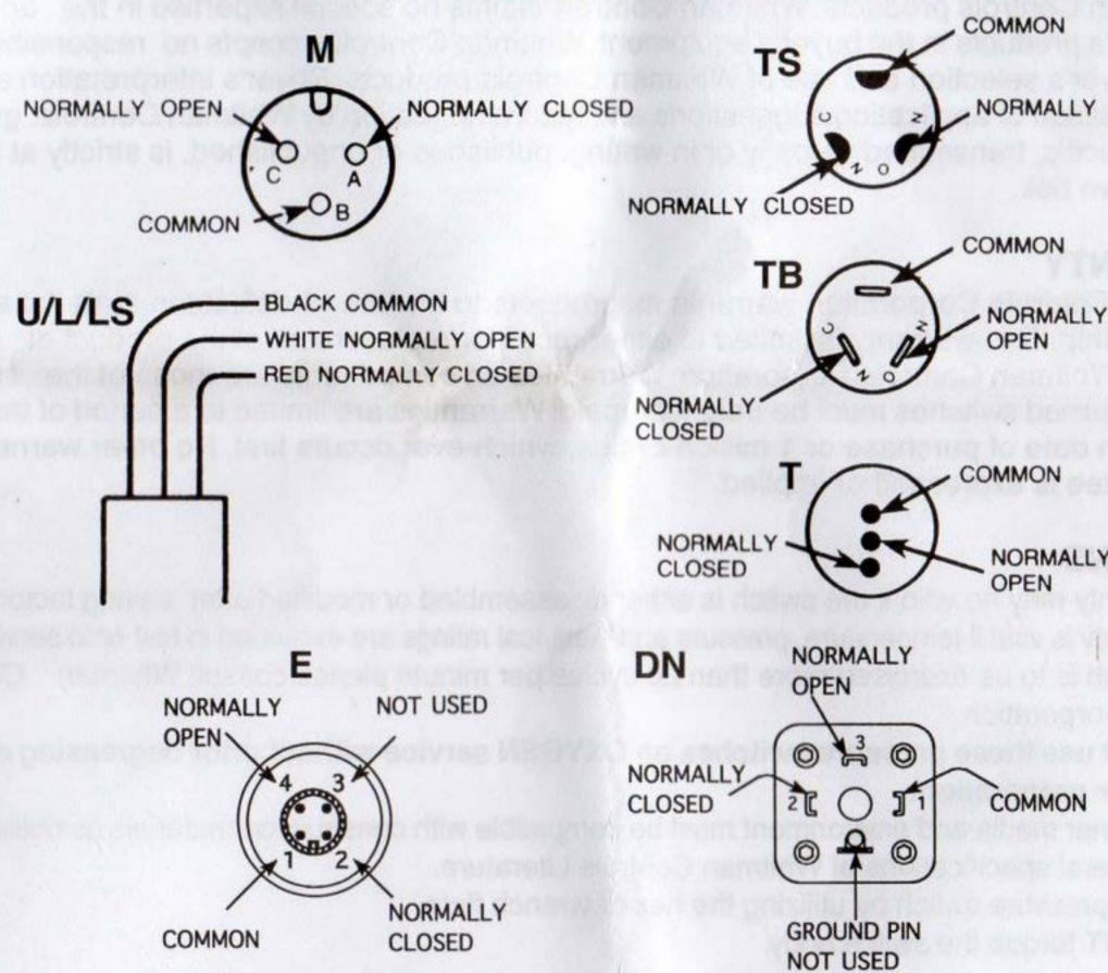
\*Vacuum Switches: Normally Open & Normally Closed are reversed
