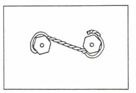
Safety wire should be run in a tightening direction only, 6 to 12 twists per inch.
