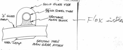
2 plies of BID at 45° wraping around the 5/8" steel tubes, over the small carved piece of urethane foam, and down onto the gear leg. Make sure it also laps onto the inside face of each glass tab.
