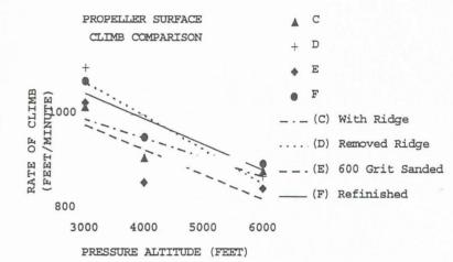
The above graph shows the stepped rough leading edge increased ROC (Rate of Climb) by 33 FPM. After sanding the whole blade with 600 grit paper, 60 FPM was lost. Finishing the prop to a high gloss, gained 70 FPM. The refinished prop produced about 5 knots extra at all altitudes. One may conclude a prop should be kept in high gloss condition for best performance.
