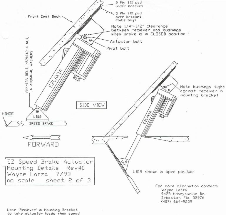
Note 'Reciever' in Mounting Bracket to take actuator loads when speed brake is extended. The compressed state, as shown, is to be typical when the brake is retracted.
