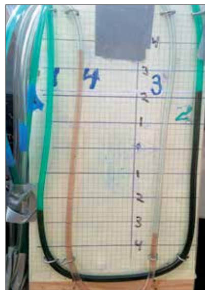
Figure 1: Two manometers were used for testing. One measured the pressure difference between the static pressure and the plenum above cylinders 3 and 4. The other measured the difference in pressure across cylinders 1 and 2.
