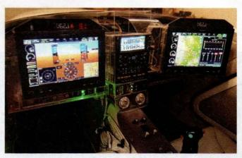
It is of amazing benefit to work on a panel that is transparent. Reaching behind and drilling holes, placing screws, and connecting wires is easier, because you can see right through the panel to everything you touch. I have learned much in the process of materials handling with cutting, drilling, and bending, having a sizable stack of failed plastic to prove it. It is difficult to photograph something that is transparent, however.
