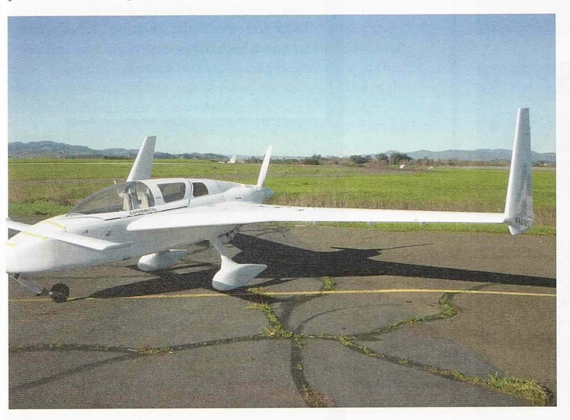
built per plans with one major exception: It's powered by a 1991 Mazda 13B fuel-injected, water-cooled, rotary engine driving a three-blade composite propeller, which I built. Tracy Crook, of Real World Solutions Inc., supplied the RD-1B gear reduction drive, the EC3 EFI ignition controller, and EM3 engine monitor.
