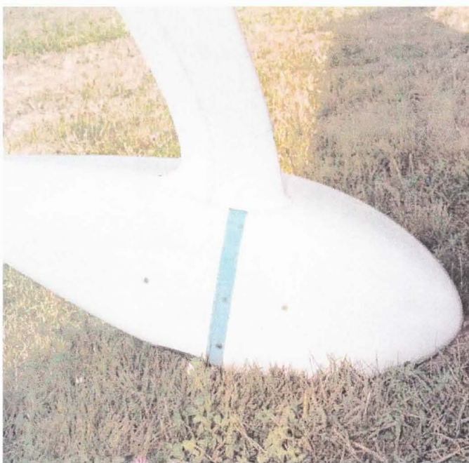
Figure 11: More zig-zag tape on the wheelpant trips the boundary layer there as well.
