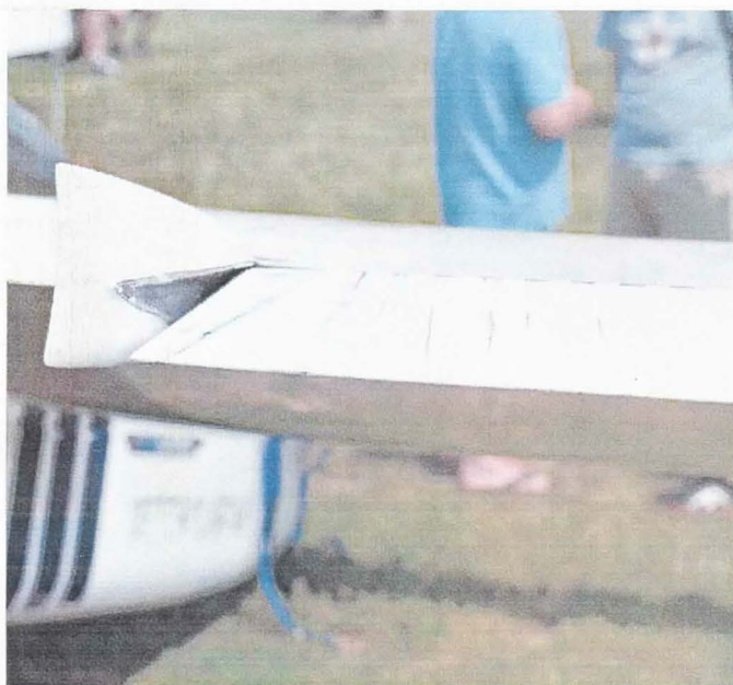
Figure 7: Aerodynamic improvements to the ailerons.
