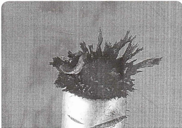
Running a mechanic's magnetic pickup tool around in the drained oil is a good idea for any engine, but particularly for Continental engines where the suction screen cannot be inspected.
