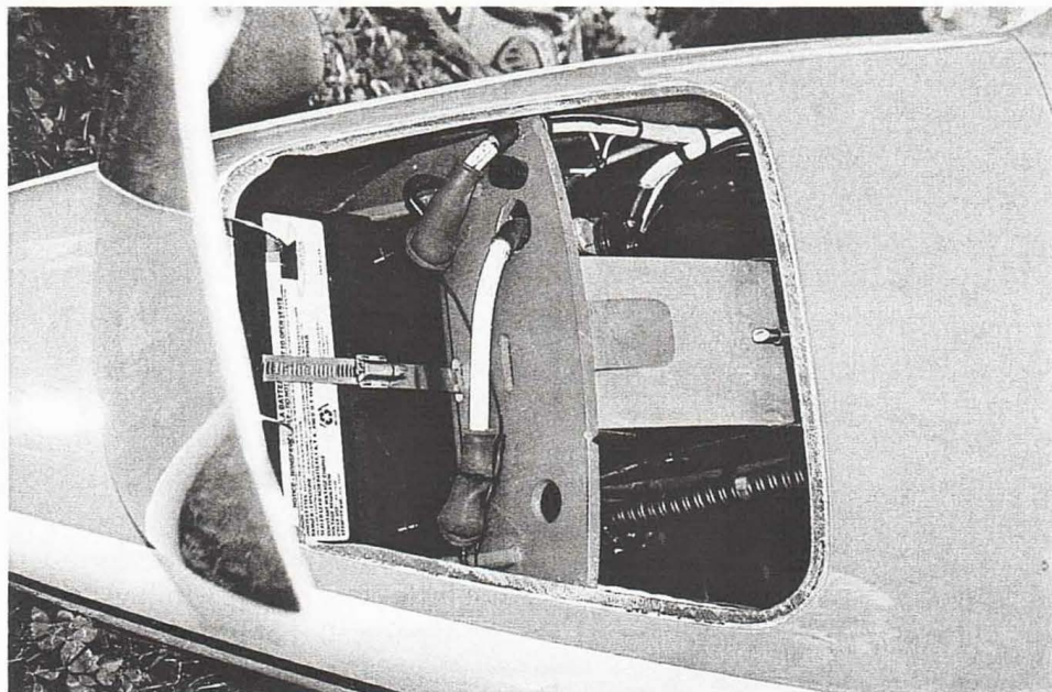
The extended nose of N14DL provided room for the aircraft's battery, a heater and fire extinguisher.
