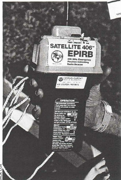
Dave Lind's Satellite 406 Emergency Position Indicating Radio Beacon (EPIRB), which he bought for use on his flight to and from Hawaii in July of 1996. It carries a code that identifies the airplane and pilot/owner.
