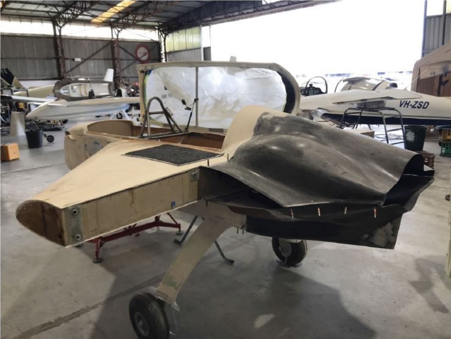
ABOVE: The aircraft has been modified in many ways, including additional perspex viewing ports, wider canopy, RAM air intake, improved landing gear leg fairings and a bespoke fuel system for long flights.
