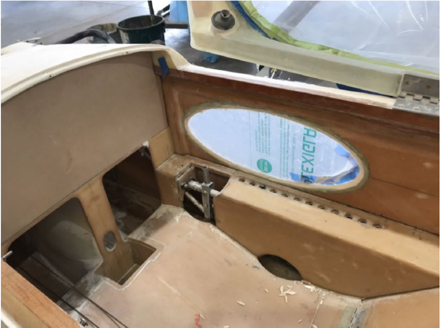
ABOVE: Dave has made countless modifications, including these perspex sight windows that improve visibility.
