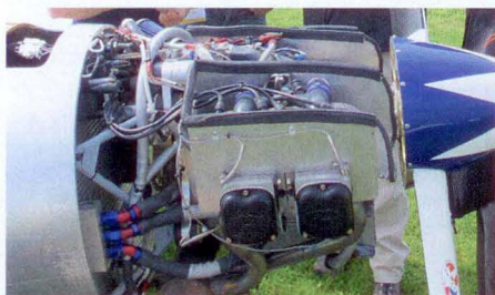
The installation of the aerobatic UL260 ISA is extremely neat and tidy
