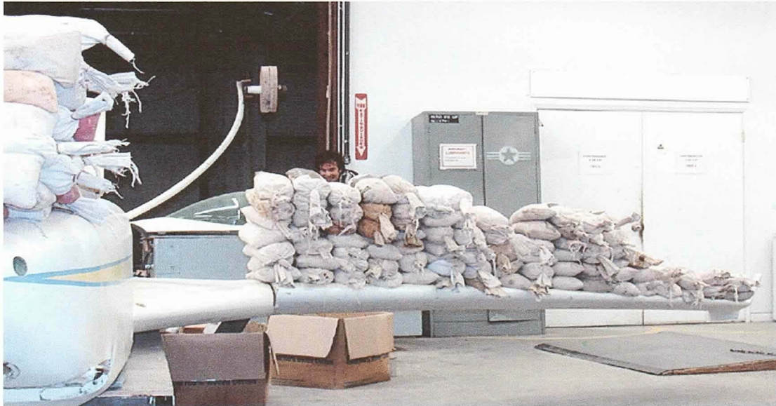
The left wing shown one instant before it failed catastrophically at 7 'Gs' Note the leading edge of the wing mismatched with the fuel strake as it fails!
