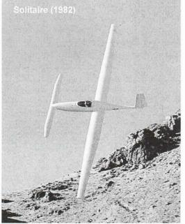
In 1982, Rutan built a single place self-launching sailplane. As usual it has a canard - a hall mark of Rutan's designs. A 23hp KFM 107E Retractable engine located in the nose driving a prop gave it the self launching capability. With a span of nearly 42' it had a glide ratio of 32:1. Solitaire sailplane was the winner of a contest by the Soaring Society of America. to make soaring more accessible by removing the need for the tow plane. The aircraft worked very well, but few were ever built.
