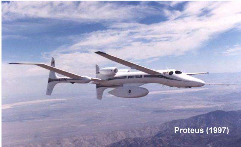
In 1997, Rutan designed a high-altitude, long endurance aircraft for telecommunication, atmospheric sampling & Earth monitoring science missions. Named Proteus after the mythological Greek sea-god who could change his appearance at will, it features an unconventional tandem-wing, twin-boom configuration with two rear-mounted turboprops on the fuselage. Its
