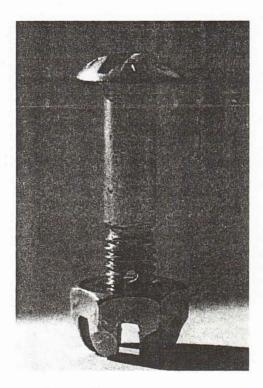
A variety of head markings are used, the most common being the sixpointed raised asterisk (or raised cross) of the AN bolt. All aircraft bolt heads have a raised marking of some sort. It may include the manufacturer's initials as well as the cross or asterisk, or it may—in the case of a special bolt—simply bear a part number or the letters 'SPEC.'
