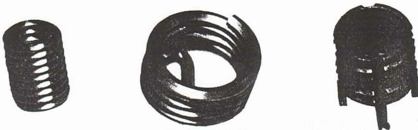
Figure 5. Wire-type thread inserts (left) can be made to lock by distorting a section of the thread form (center). Other inserts, such as the elastomeric device at right, resemble the locking portion of a prevailing-torque locknut.
