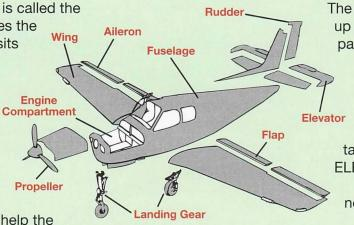
The tail that sticks straight up like a shark's fin has a part called the RUDDER. The rudder helps turn
